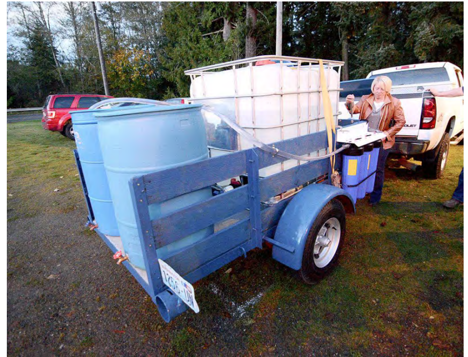
Figure 42. Case study: Joyce Emergency Planning and Preparation's Water Treatment System filters untreated water using chemical and physical water purification. See page 196 in the Appendix.
