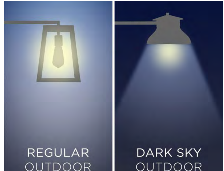
Figure 29. An unshielded light fixture and a fully-shielded light fixture.
